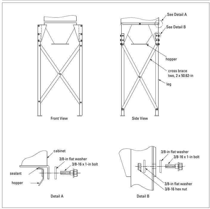
Hopper to 55-Gallon Drum Assembly (Size 90 hopper is welded to cabinet)
