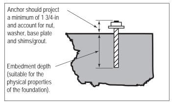
Typical Foundation Anchor for Collectors With Hopper and Leg Assemblies
