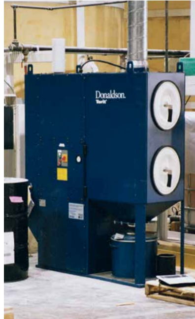
DFO on Paint & Pigment 1,200 cfm (2,038 m 3 /h)
