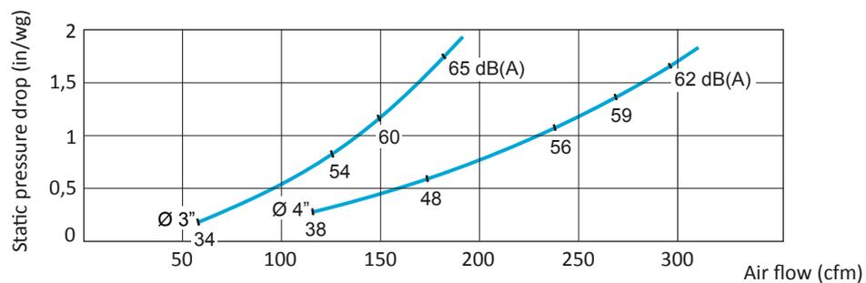
The static pressure drop is measured in accordance with ISO standard 5167-1. The noise level is measured according to ISO standard 3741.
