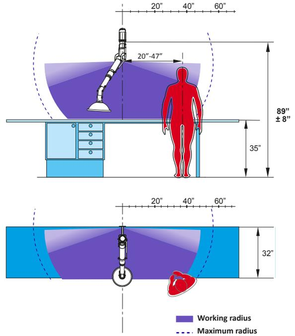
To optimize the usability of the extractor, the above mentioned mounting heights, and sideways displacements from the workplace, are recommended.
